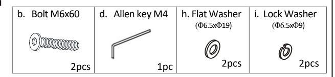
• Attach Support legs (5) to Centre rail (4) with bolts (b), Flat Washers (h) and Lock Washer (i).
